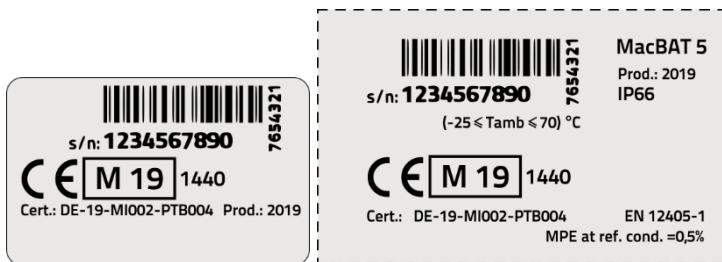
Figure 10. Nameplate placed on front door of the device (left – plastic housing, right – metal housing)
